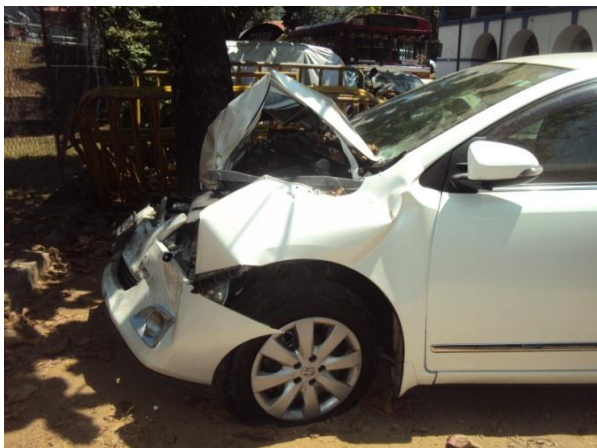
Figure 2: Extensively collapsed crumple zone.
